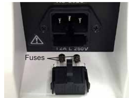
Figure MM-05 Replace Fuses
