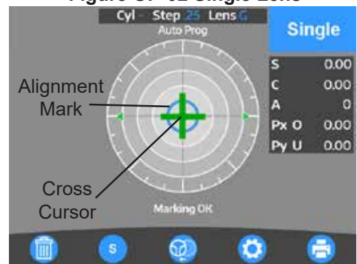
Figure OP-03 Alignment
